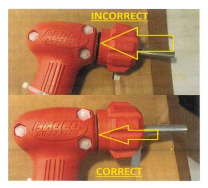
• The collet should be fully seated to the bottom of the collet flange, approximately 1/16 of an inch above the top of the torch head.
