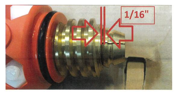
• If the collet is too high, remove the collet nut, the collet and the collet washer. Using the 5/32" hex key provided, remove the flash arrestor.
