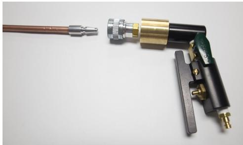
And specific to the Broco quick release, the coupler is fairly large making it easy to grip and twist while wearing gloves. And because it is twist-lock (twisting in the same direction as tightening so the collet nut doesn't accidentally loosen) it doesn't have the roller balls under the collar so won't get messed up by dirt or corrosion as easily.
