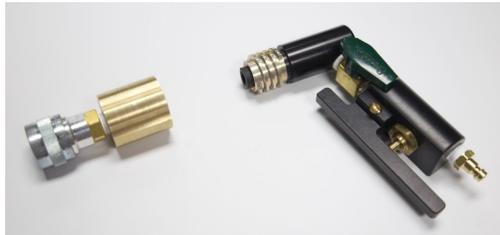
Advantages for our quick connect setup are speed, positive engagement (a quick click and the rod is locked into place), no oxygen leaks, and easy removal (no more pulling a hot rod stub from the collet).
