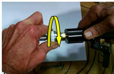
11. To remove the cutting rod stub, twist the sleeve of the coupler clockwise. (The same direction as if you were tightening the SNAPNUT.) Fitting should fall out.
