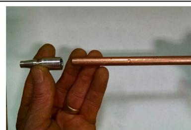
6. 'SNAP' rod fittings can be pressed onto the recessed end of the cutting rod by hand. Select a fitting of the appropriate size for the cutting rods being used. (3/8" or 1/2")
