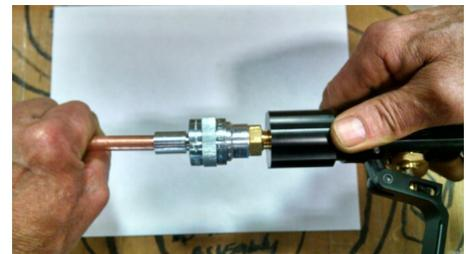
10. Press the rod tip firmly into the quick connect coupling until it is felt to lock in place.
