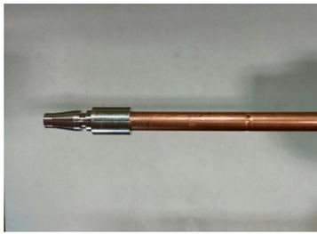
7. Place the 'SNAP' fitting on to the recessed end of a cutting rod and press until it can't go any farther.
