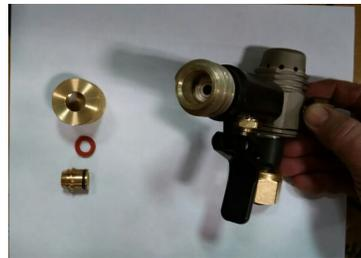
2. Remove the collet nut, collet and collet washer.
