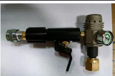
5. Screw the nut onto the torch and hand-tighten securely.
