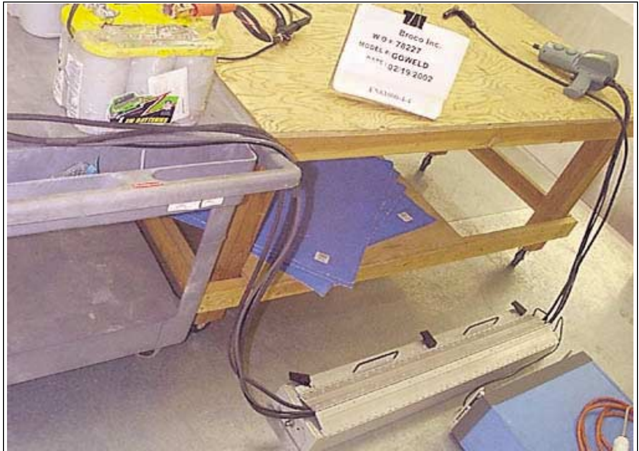
Electrical Fast Transient Burst - Power Lines
